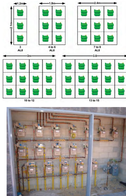
Figure 36 AL8 Gas Meter Groupings
