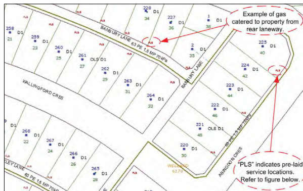
Figure 3 Plan Showing Gas Mains and Pre-Laid Service Locations
