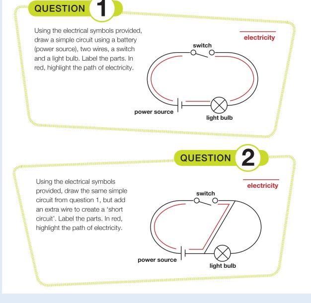
Electricity travels through some materials better than others. Conductors are materials that allow electricity to travel through them. Insulators resist electricity. You will investigate these two types of materials in the upcoming questions.
