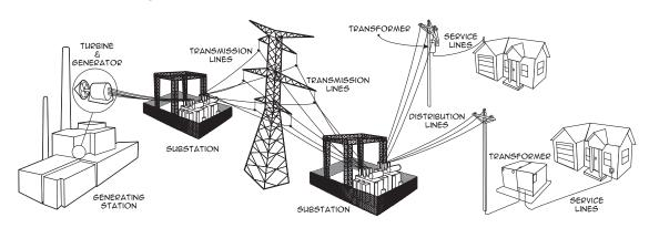
The ground is used as part of the electric system. Electricity looks for a path to ground throughout the circuit. Part of ATCO's job is to keep electricity away from the ground until it is delivered to customers and used. The electricity will arrive where it is needed unless some conducting material touches the wires along the way and provides a path for the electricity to get to the ground.
