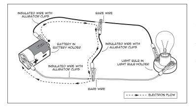
b) Explain to students that the battery will be 'shorted' and will heat up because of the high current flow. The current flow is high because there are no parts of the circuit to resist the electricity (e.g., light bulb).
