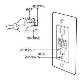
ground wire, so the circuit is ungrounded. In this case, if a hot wire touched a conducting material and a person touched the material, the person would become the path to ground.
