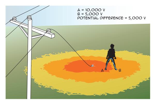
If electric wires are knocked down during an accident or in a storm, assume that the wires are still energized. Everyone should stay at least 10 m away from the wires. ATCO should be contacted to turn the electricity off. The line is safe only when an ATCO employee or emergency responder indicates that it has been turned off.
