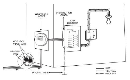
These wires are insulated from each other. The hot and neutral wires form the electric circuits for each light, outlet or appliance to which they are connected. The hot wire carries electricity from the generating station. The neutral and ground wires are connected together and provide a return path for the electricity outside the house.
